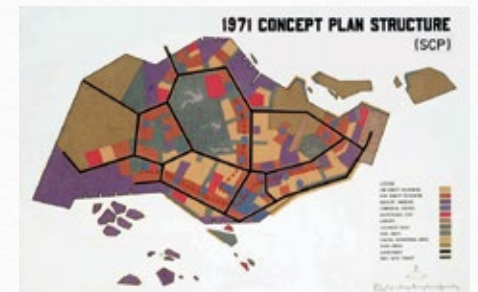
The 1971 Concept Plan set out broad principles to develop new housing towns, industrial estates, transport infrastructure, and recreational spaces across the island via a ring structure of satellite towns around the central water catchment.
